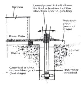
The compressive strength of the grout must exceed  $55 \text{ N/mm}^2$  at 7 days and  $65 \text{ N/mm}^2$  at 28 days.
